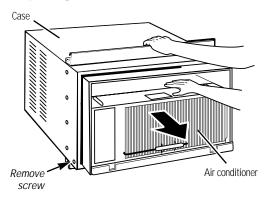
Slide the air conditioner out of the case by grasping the rear of the evaporator cover and pulling forward while bracing the case.
